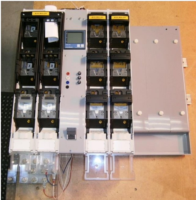
BBS8-1300IUMG with 1250 amp isolator, internal MDI, Phasing sockets, street light fuse carrier at the bottom & 3 spare 100mm ways.
