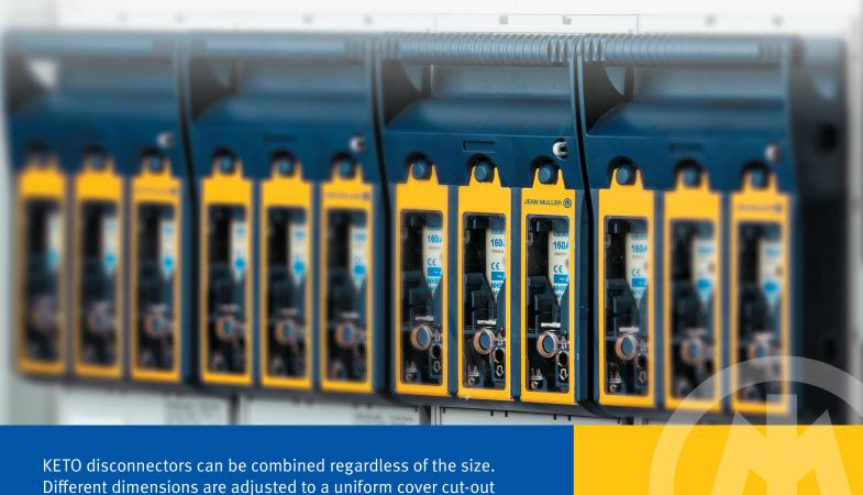
KETO disconnectors can be combined regardless of the size. Different dimensions are adjusted to a uniform cover cut-out with the available components for touch protection. Many functions are integrated across all construction sizes, e.g. four cover support levels at 32, 60, 70 and 90mm above top of busbar. This ensures an optimal system integration. Version for baseplate mounting, busbar and DIN rail mounting offer the suitable solutions for each application.
