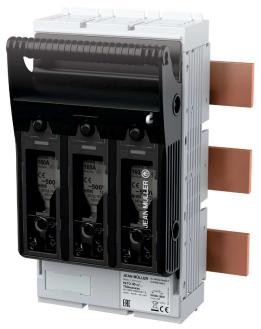
KETO disconnectors can be combined regardless of the size. Different dimensions are adjusted to a uniform cover cut-out with the available components for touch protection. Many functions are integrated across all construction sizes, e.g. four cover support levels at 32, 60, 70 and 90mm above top of busbar. This ensures an optimal system integration. Version for baseplate mounting, busbar and DIN rail mounting offer the suitable solutions for each application.
